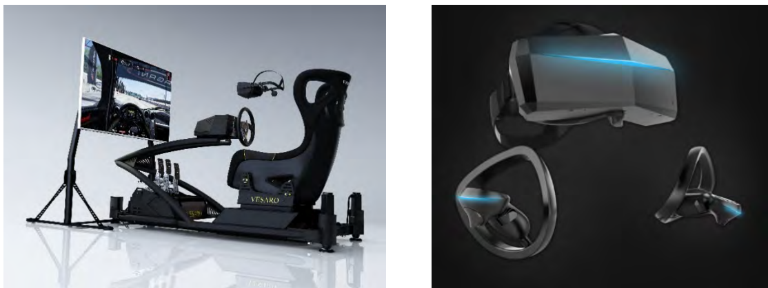
Figure 6: Shows the Connected Places Catapult's driving simulator with D-Box motion platform and the Pimax 8K plus VR headset that has a 210° Field of View.
