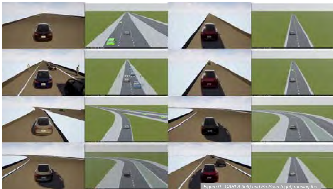
Figure 9 - CARLA (left) and PreScan (right) running the same scenarios generated by the VeriCAV framework.
